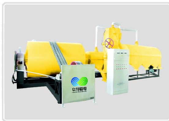
This machine is specially designed for quartz- making field for glass industry. It is composed of mill, sieve (for different size product), coarse material- returning system, and dust- collecting system. And you can get the product from different sieve with size 60- 120 mesh for glass industry. The size for powder material coming from dust collector is about 300mesh (you can use this for other business).
